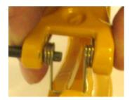
Place the latch, pin and spring in correct position as shown in the pictures.
