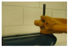
Drive the coiled pin through the assembly with a hammer. Take care that the coiled pin is fitted in both sides of the spring coils.
