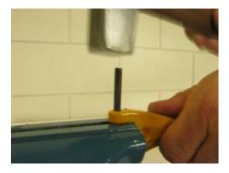
There must be enough length of the coiled pin inside the latch to put the coils of one side of the spring on.
