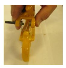
Secure this position in the hook with a pin, this pin should be smaller that the coiled pin.
