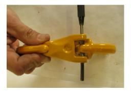
Put the assembly (including the positioning pin that is not shown) on a solid mass.
