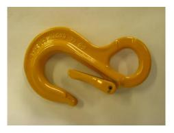
Remove the coiled pin with a well fitting pin driver. Please make sure that there is space for the coiled pin to exit the latch of the hook.
