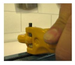
Make sure the pin is completely assembled into the latch. After assembling test if the latch is functioning correctly.
