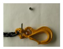
The pin must be driven trough the parts with a hammer.
