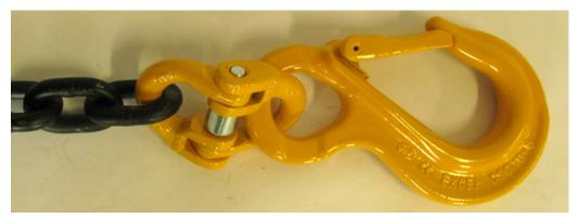
The pin is kept in place by the bush. Check the correct position (half links, pin, bush) and the locking of the components. Make sure the connecting link (both half links) can hinge freely.
