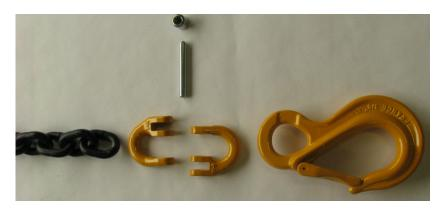
Make sure you have all the correct components to assemble the chain sling.
