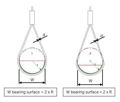
To explain the ratio between the radius of the bearing surface and the width of the crown see below diagrams:
